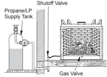
Figure 22 - Checking Gas Joints for Propane/LP Gas Fireplace
